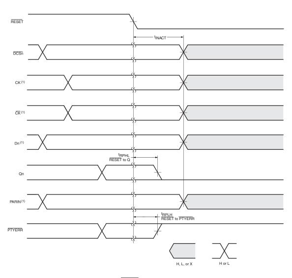
Figure 6 —  $\overline{\text{RESET}}$  switches from H to L
