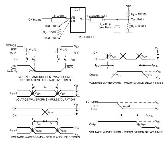
Figure 6 — Parameter Measurement Information (V<sub>DD</sub> = 1.8V±0.1V)
